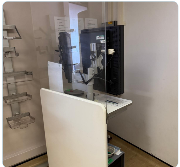
Operator workstation and radiation shield
